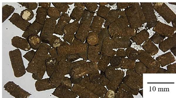
Fig. 1. View of 4 mm diameter granulated manure pellets
